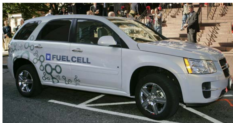
Fuel-cell-powered Chevrolet Equinox
