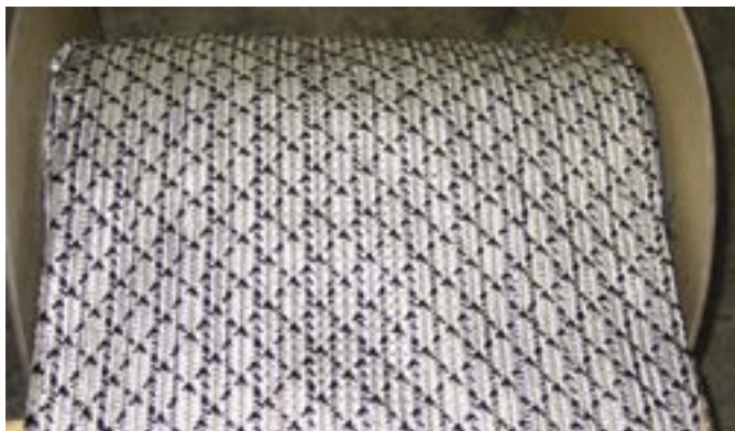
Fig. 2: Photo of the triaxially braided HFRP fabric (THD system)
