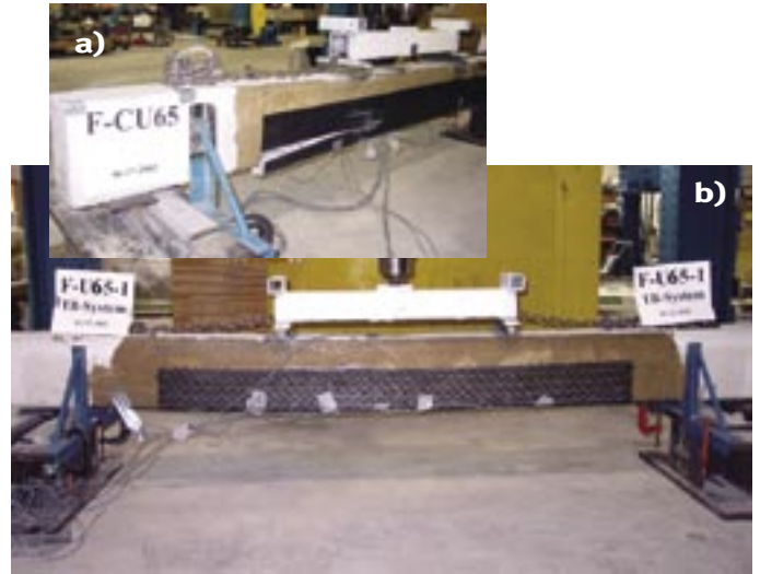
Fig. 7: Failure of two identical beams strengthened in flexure using two strengthening systems: a) carbon fiber sheet strengthening of Beam F-CU65, which was identical to Beam F-U65-1 except that it was strengthened with a uniaxial CFRP sheet that had a similar rigidity to that of the triaxially braided fabric system used in Beam F-U65-1; and b) triaxially braided fabric strengthening (Beam F-U65-1)
