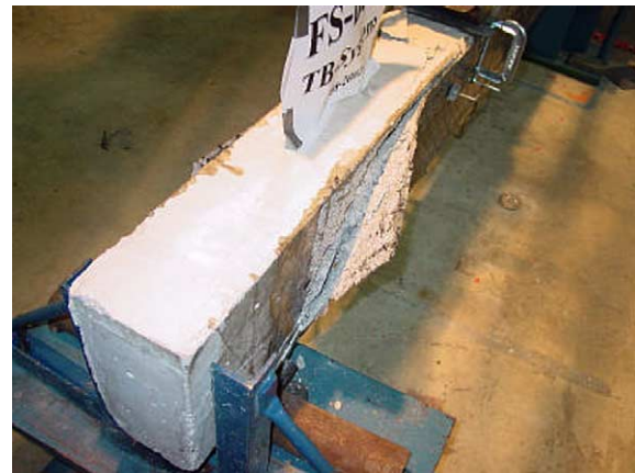
Fig. 12. Failure of beam FS-B3U.
