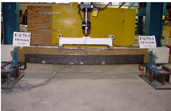
Fig. 10. Failure of beam F-U75-1.
