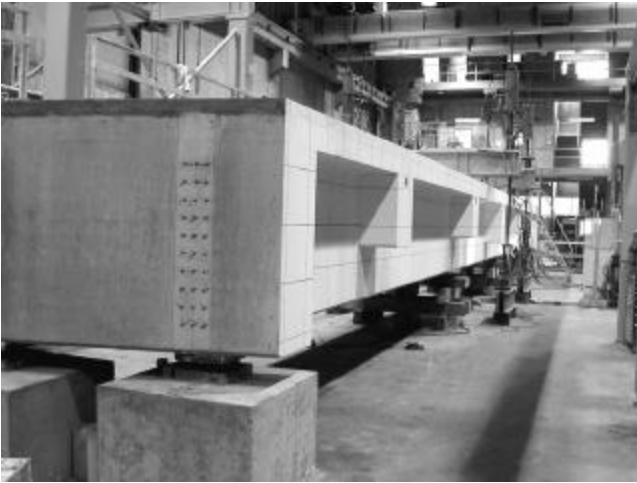
Fig. 4—Test setup for flexural loading.
