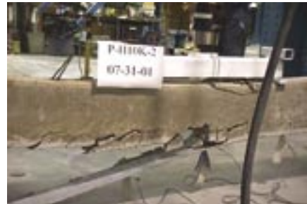
Fig. 4: Ultimate load failure of a beam strengthened with CFRP plates and subjected to 10,000 h of 100% humidity
