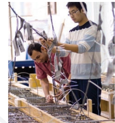
Lawrence Tech students prepare a prestressed concrete bridge beam for a research project sponsored by the National Science Foundation.
