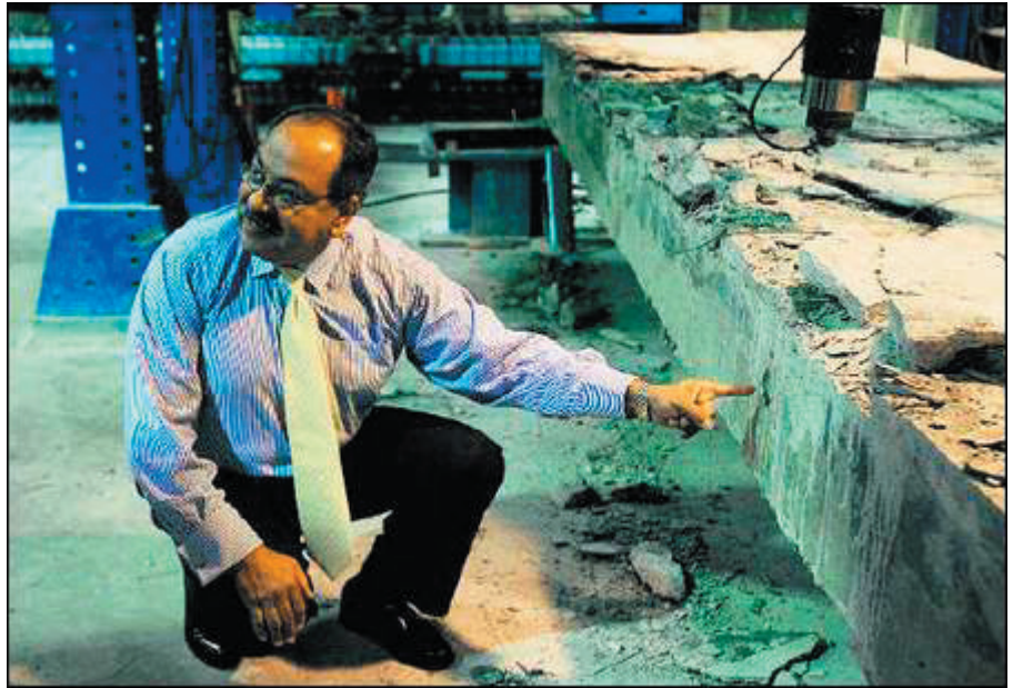
Nabil Grace, a professor and chairman of Lawrence Technological University's civil engineering department, oversees classroom testing on highway structures July 20. The research could lead to bridges being built with a carbon-fiber reinforced polymer instead of steel.
