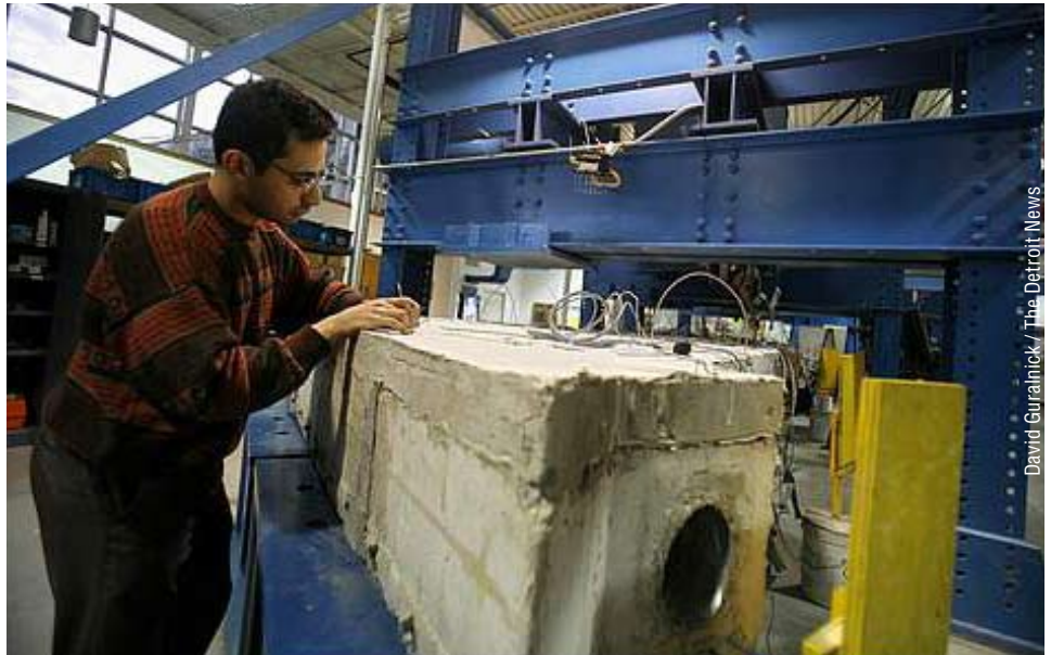
Civil engineering student Eslam Solimena is testing carbon fiber rods, seen as a more durable component for future bridges.
