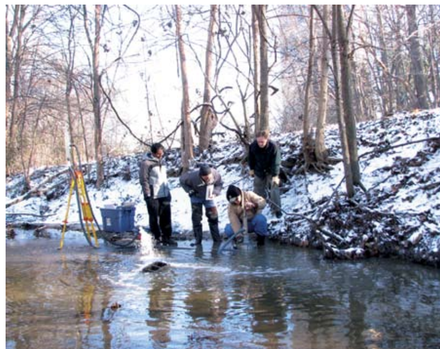
The Rouge River tributary adjacent to the Engineering Building was a good place to demonstrate equipment that measures the effect of “scour” erosion. Assistant Professor Hiroshan Hettiarachchi (L) and Associate Professor Don Carpenter (R) have received a Michigan Department of Transportation grant to improve the ability to predict the effect of such scouring on bridges.
