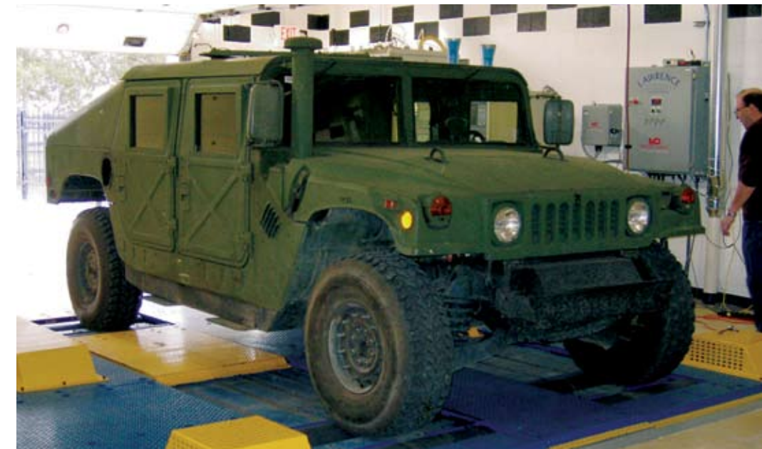
Mark Schmidt, a lab technician in the Department of Mechanical Engineering, puts a Humvee through its paces on Lawrence Tech's four-wheel-drive chassis dynamometer as part of a research project for TARDEC.
