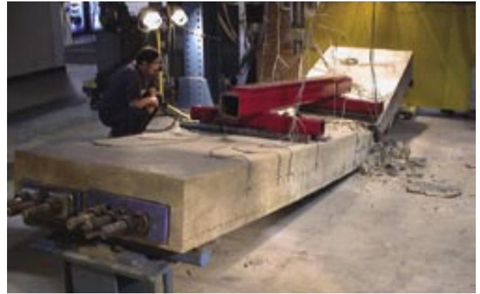
Fig. 3: Shear failure of box beam M2 with S A stirrups
