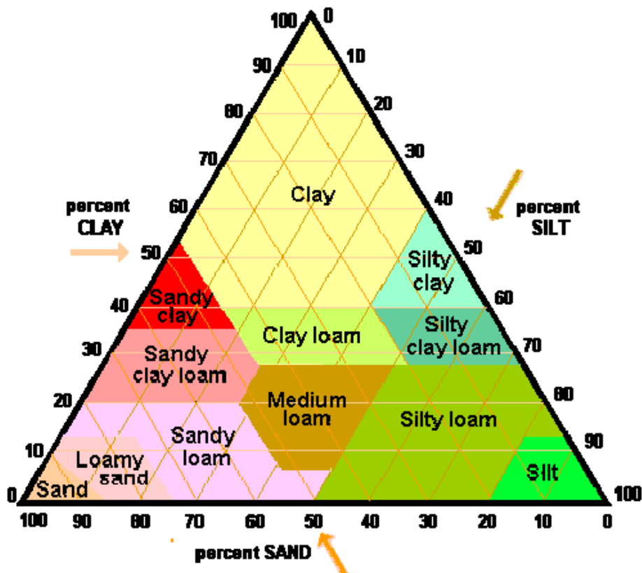
Figure 1: Soil Classification Triangle (Reprinted with permission from the Idaho Association of Soil Conservation Districts)
